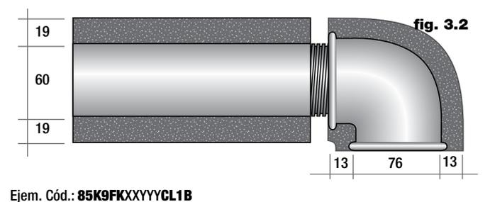
**4) CURVAS EN POLIPROPILENO NORMA 1/A SIN PERDIDA DE ESPESOR**
