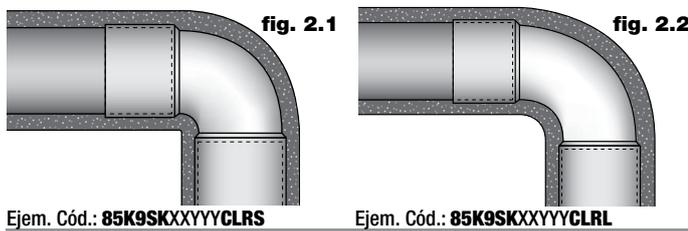
**CURVAS EN COBRE "PRESSFITTING" A RADIO LARGO (figura 2.2)**
